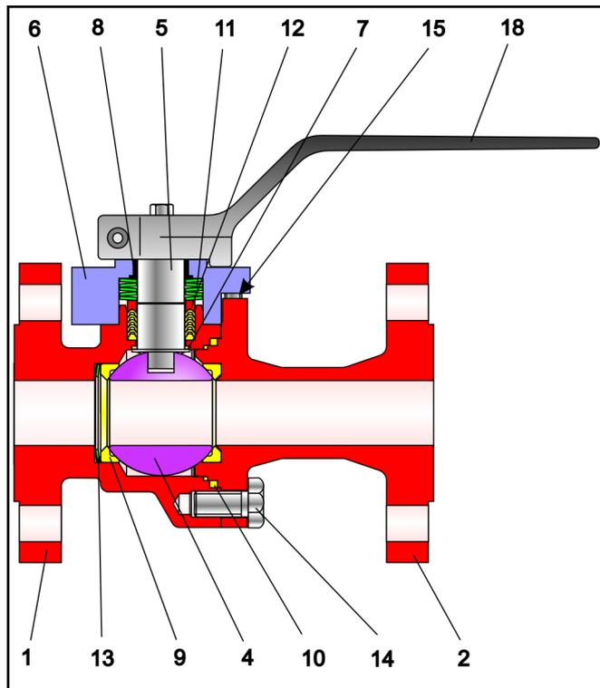
Fig. 3 – Sectional diagram of Series 26a Ball Valve
