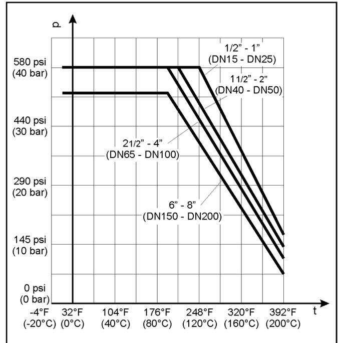
Fig. 6 - Pressure-Temperature diagram
